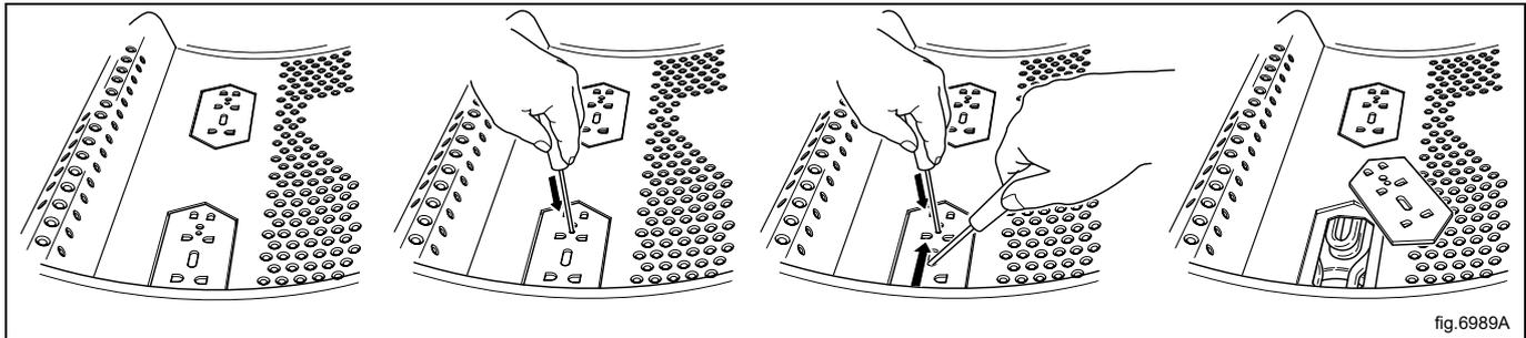
Remove the core element/elements and clean the elements. If the elements are very dirty, it may be wise to remove the elements from the drum when cleaning them
